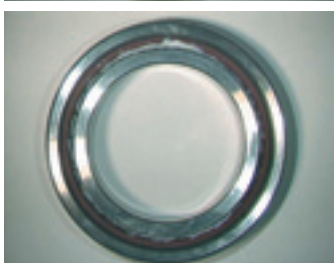
Photo. 6.1 Filling grease into angular contact ball bearing
