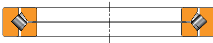
Fig. 24. Type TXR crossed roller bearings.
