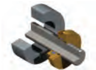
Figure 14: Seal Installation on Shaft
