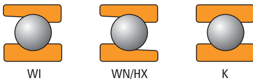
Fig. 21. Angular contact spindle bearing types.
