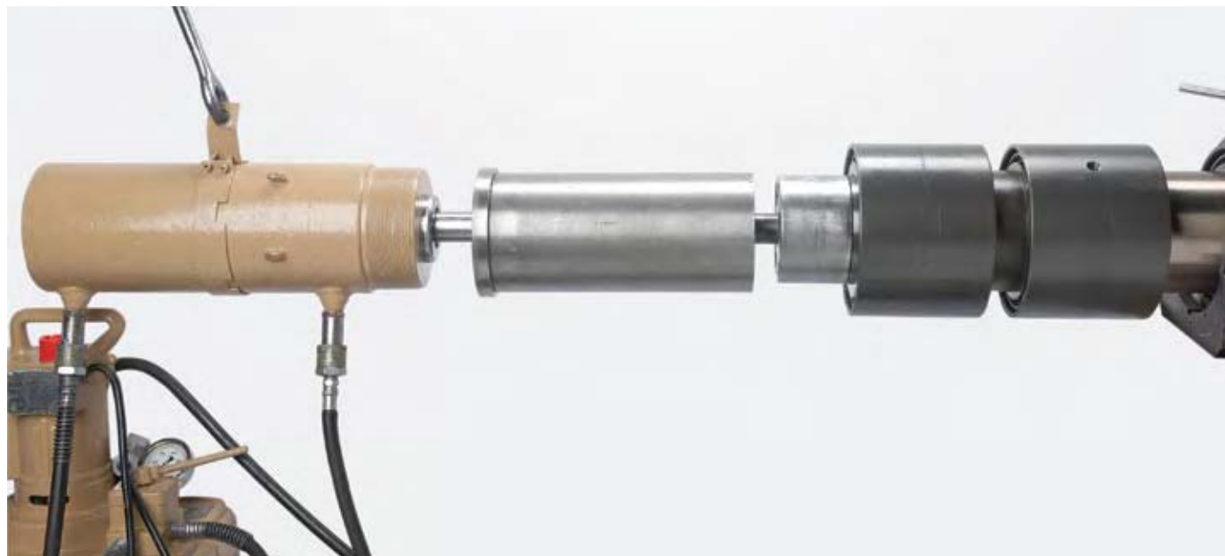
Fig. 28 Tooling used to push bearing onto shaft
