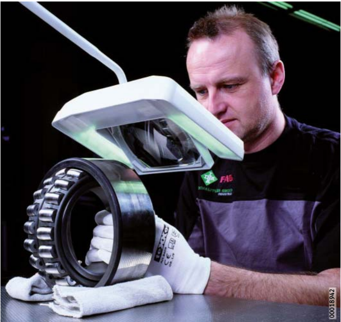
Figure 6 Bearing examination by Schaeffler reconditioning specialists
