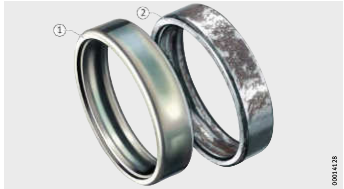
Figure 7 Bearing rings after the salt spray test
