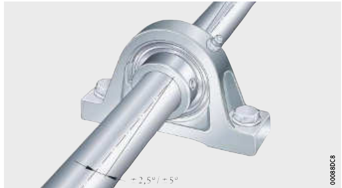
Figure 5 Compensation of static shaft misalignment
