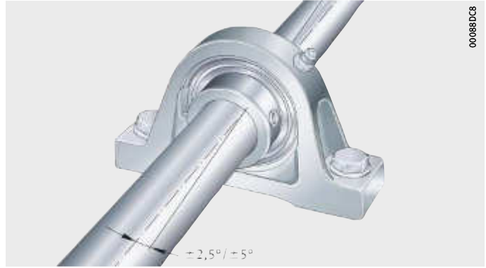
Figure 1 Compensation of static shaft misalignment
