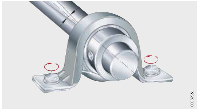
Figure 12 Screw mounting the housing finger tight
