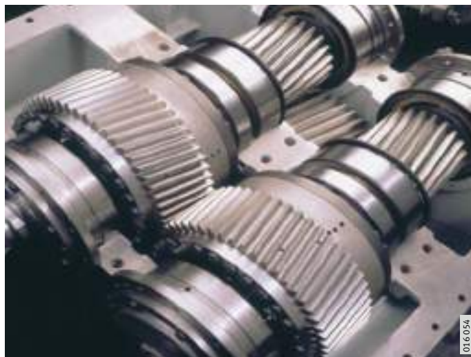
Figure 5 Rolling bearings in a cylindrical gear unit
