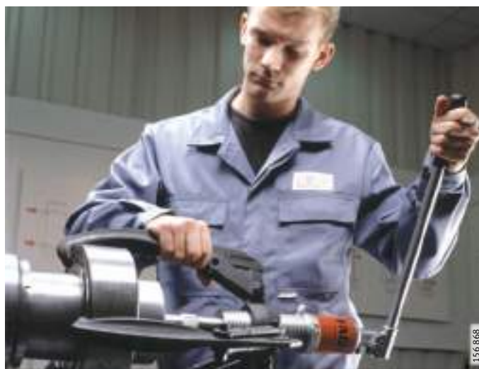
Figure 1 Dismounting of a bearing using a hydraulic extractor
