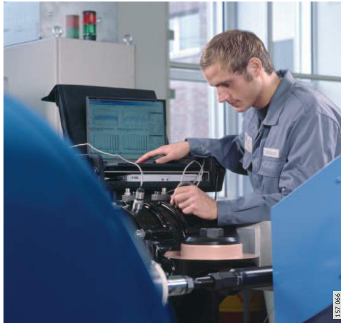
Figure 9 Condition-based rolling bearing monitoring using Bearing Analyser
