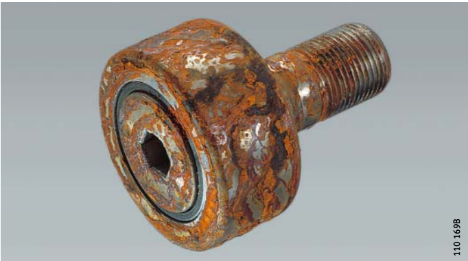
Figure 1 NUKR52 without coating after salt spray test
