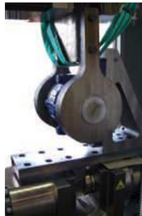
Load test: Tensile test parallel to mounting surface. During the test phase, SNC housings are loaded to their limits.
