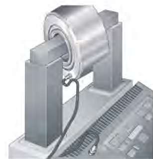
Heating with an induction heater
