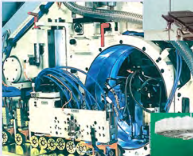
Franke bearing assembly in a welding machine. High radial and axial accuracy for best welding results.
