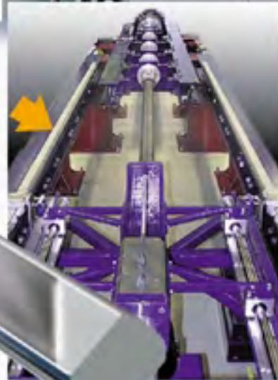
Coupled roller guides in a crash test application. The sledge moves with high dynamic acceleration.
