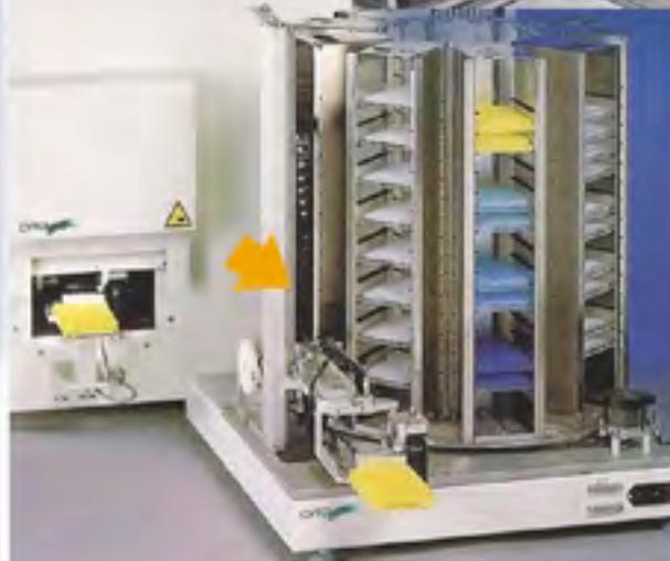
Aluminium roller guide in a climate chamber. The guide system has to face temperatures from 0 to 90° C and humidity of 90%.
