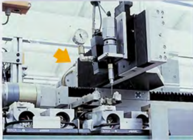
Franke linear tables in a production line for motor housings. The double axis unit moves a dosing pin for sealing material which is applied to the contours of the housing parts.
