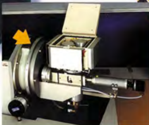
Franke rotary tables for positioning climatic chambers. The investigation chamber is moved along 2 axes. The silent vibration-free run guarantees troublefree measuring results.
