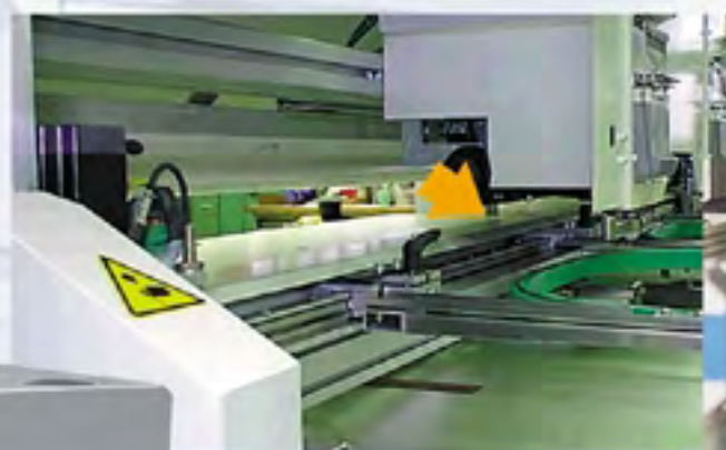
Embroidery automate with movable embroidery frames. The aluminium roller guide moves in short strokes with high frequency, thus allowing detailed embroidery patterns.
