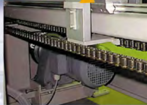
Take down pusher in a packing machine for mattresses. The rolled mattresses are pressed out of the drum with a pressure of 1.5 t. Aluminium roller guides provide the precise movement of the pusher.
