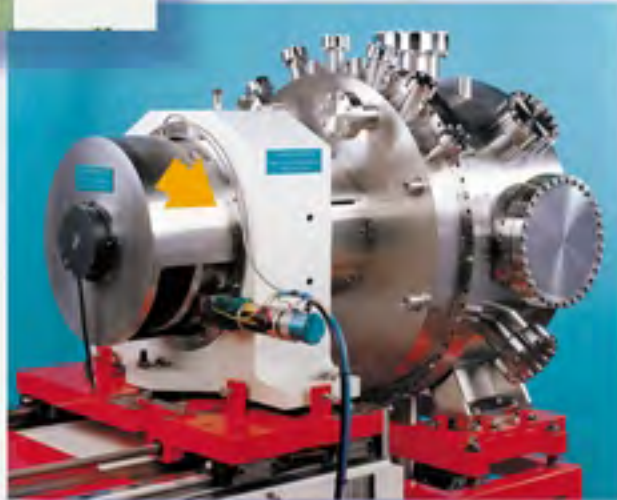
Franke rotary table in a x-ray monochromator. The heavy sample carrier is positioned by a Franke rotary table of high precision. The large center space of the rotary table facilitates easy centering of the x-ray.
