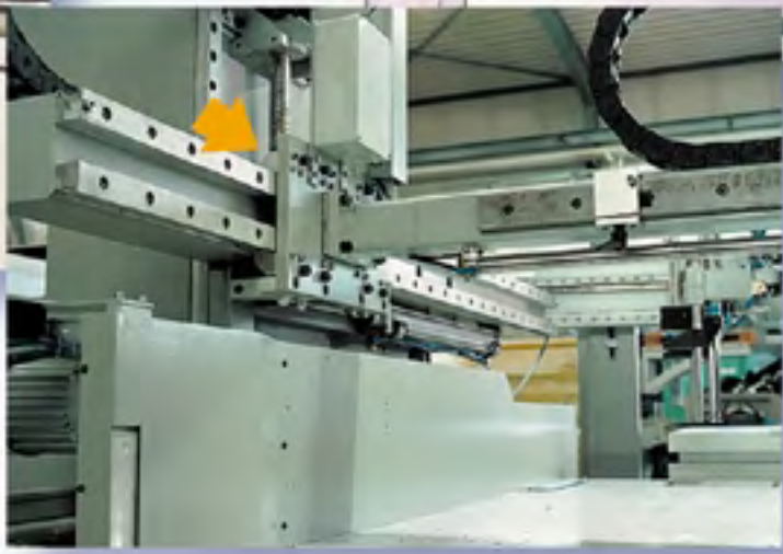
Handling device for paper stacks. The aluminium roller guides move jigs and stops reliably in permanent operation.
