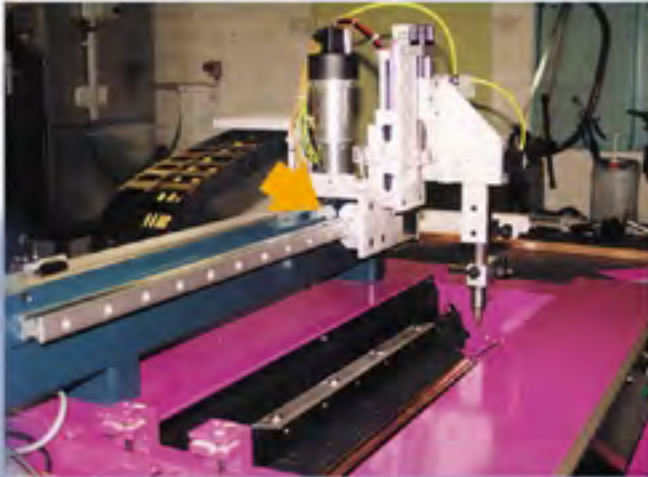
Aluminium roller guides in a welding machine. The welding head is moved horizontally with high accuracy thus enabling the machine to create small and precise welding marks.
